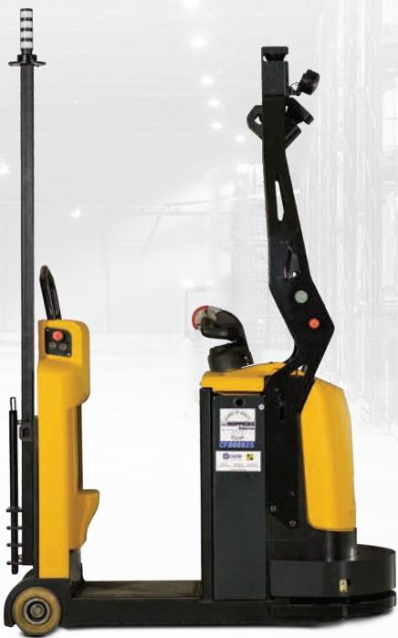
The Robotic Tow Tractor offers an autonomous solution specifically for long, repetitive tasks such as milk runs and garbage hauls with a 15,000 pound capacity rating. Tasks that typically lead to higher operator turnover, you can now retain talent by automating these mundane repetitive tasks and promote your skilled operators to more engaging, value-added tasks.
